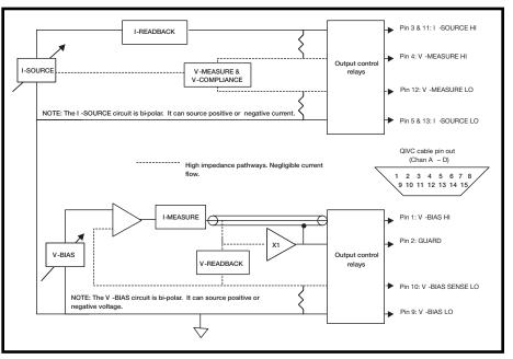
Figure 3. Basic block diagram of source measurement components of the Series 4500-QIVC cards.
